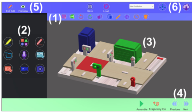
Figure 4. Main interface of the Meta-AR-App (Instructor Mode): (1) Toolbar; (2) Animation Palette; (3) Canvas, (4) Controls, (5) Edit Mode, (6) Collaboration Panel.
