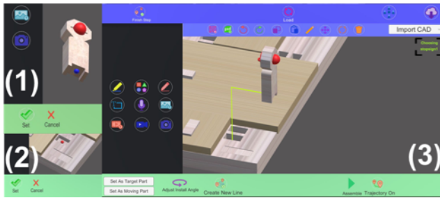
Figure 6. Creating Animation Process: (1) select start point from Object A and set; (2) select finish point from Object B and set; (3) path is generated and instructor can preview animation.
