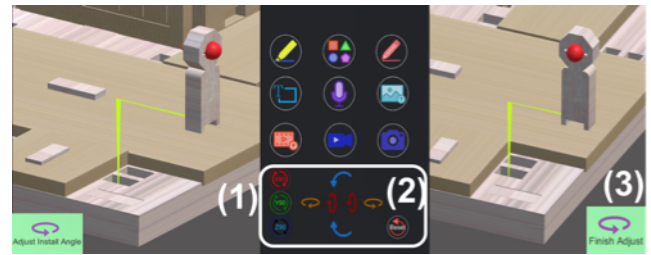
Figure 5. Angle adjustment process: (1) Object A and path have the wrong orientation; (2) Angle Adjustment tools can be used; (3) Object A and path are aligned. Sample objects from our mini smart-city user study.
